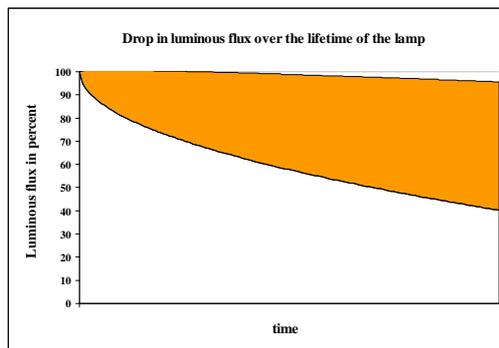
For assessment purposes this drop in light output can be taken into account by considering the luminous flux averaged over time and/or by setting a specific admissible drop value.
