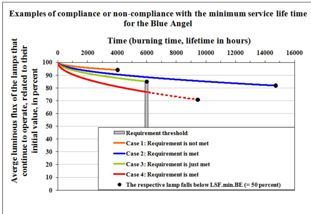
Case 1: The requirement is not met because the lamp survival factor reaches the value of  $LSF_{min.BE}$  (= 50 percent) prior to the end of the required 6,000 hours.
