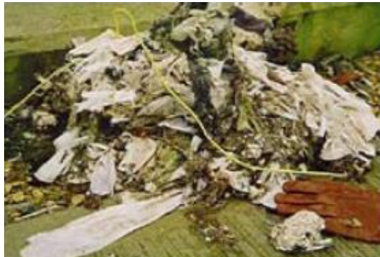
Figure 3-2: Typical material removed from a conventional 300mm discharge sewage pump
