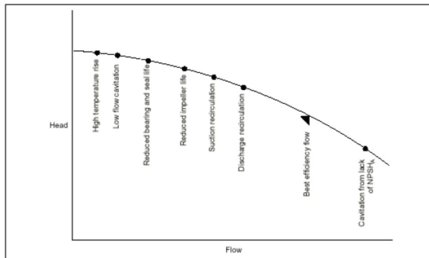
Figure 3-7: Onset of adverse effects when operating a pump away from its peak efficiency flow
