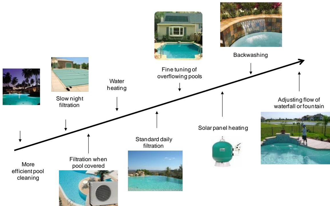
Figure 3-1: Intelair diagram indicating the variation of duties a pump may be expected to supply – Many domestic pumps will only perform filtration, heating and backwashing
