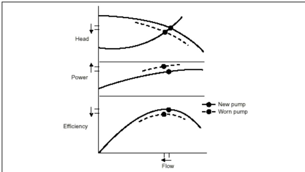
Figure 3-2: Effect of wear on pump characteristics
