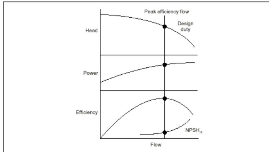
Figure 3-6: Centrifugal pump characteristics
