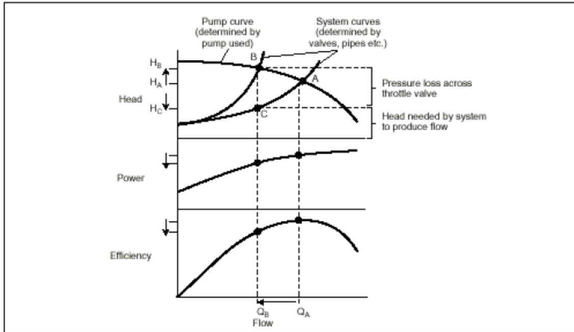
Figure 3-8: Illustration of the effect on the efficiency of throttling a pump
