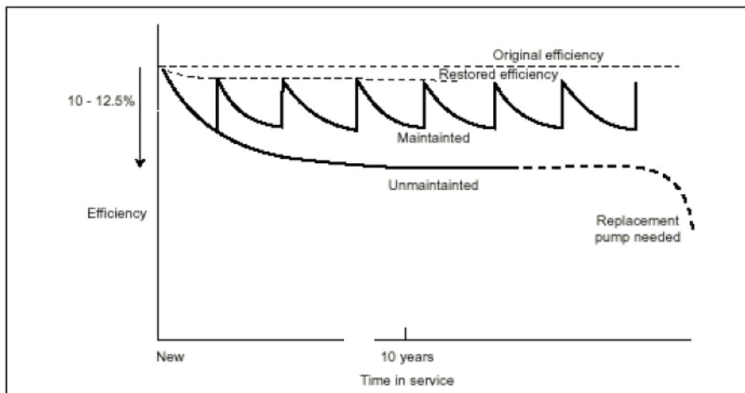
Figure 3-3: Average wear trends for maintained and unmaintained pumps
