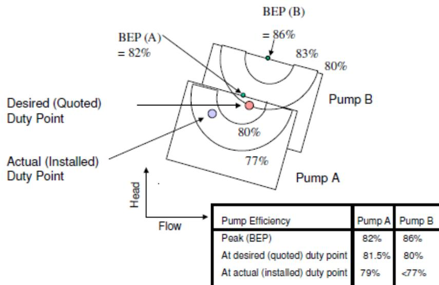
Figure 3-5: Worked example showing the importance of correct selection of a pump
