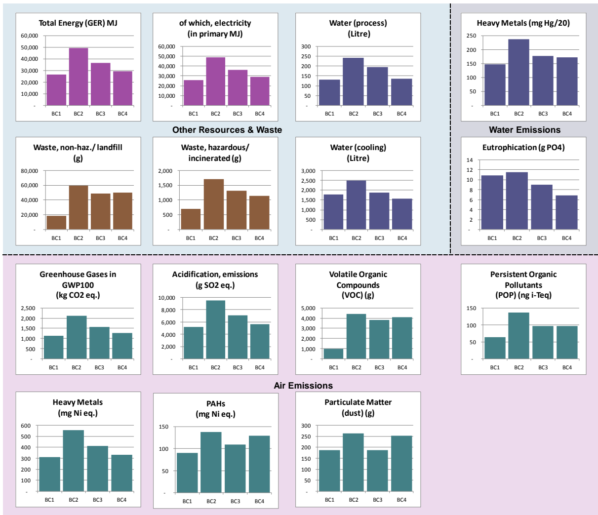
Figure 4: Results for each base case across the different environmental impact indicators (normalised by kW across lifetime)
